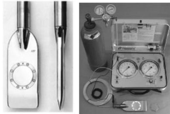
Figure 7 Flat Dilatometer Marchetti Test
